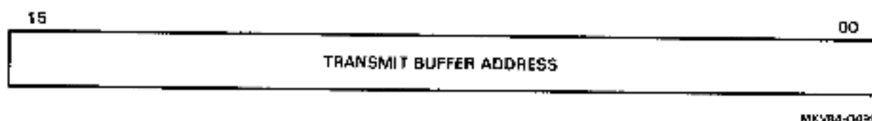
Figure 3-13 Indirect Register (IND.REG[2]<15:0>) Bit Map – Read/Write
