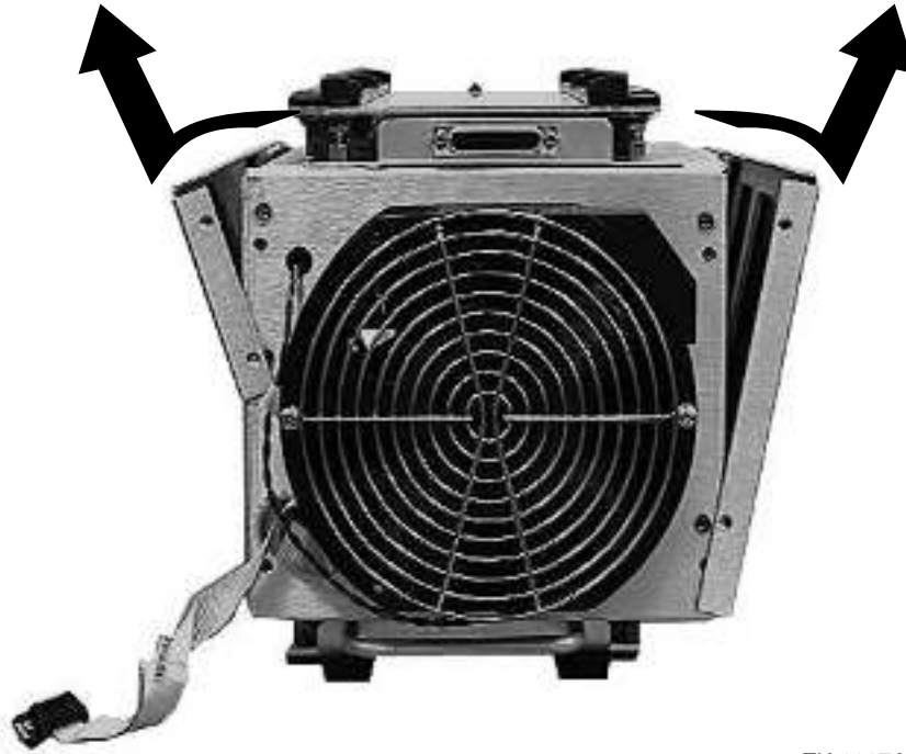
Figure 6–7 (Cont.) Side Panel Removal
