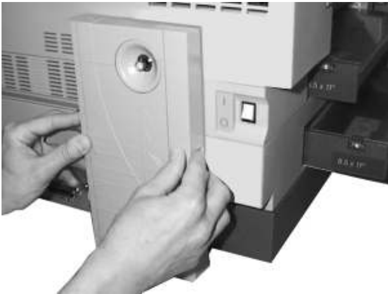
Figure 1-7 Attaching LATprint ThinWire Ethernet Interface to the DEClaser 3200
