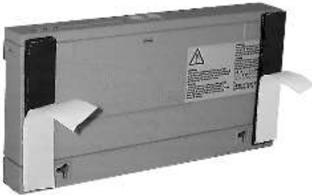
Figure 1–8 Attaching Mounting Strips to the LATprint ThinWire Ethernet Interface
