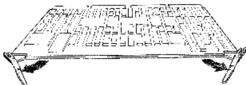
Figure 8-32 Quad-Height Module Ejector Levers
