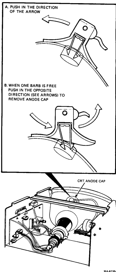
Figure 2-16 Removing the CRT Anode Cap
