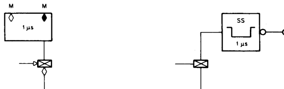
Figure 3-6 (f) Monostable Multivibrator (Single Shot)
