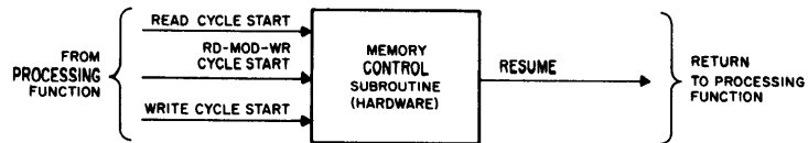
Figure 7-6 Memory Control Functions
