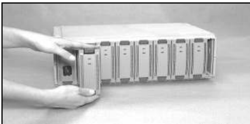
Figure 1–4 Removing an SBB from the Shelf
