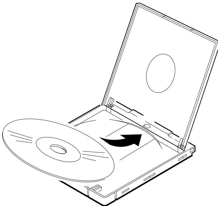
Figure 2-14 Inserting Disc Into Caddy
