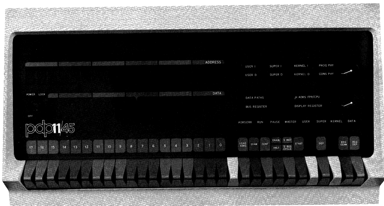
Figure 4-1 PDP-11 Switch Register Console
