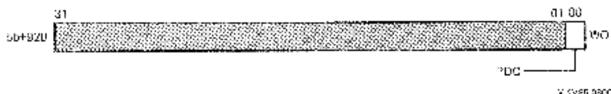
Figure 4-35 Port Disable Control Register Bit Map
