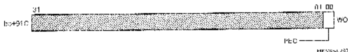
Figure 4-34 Port Enable Control Register Bit Map
